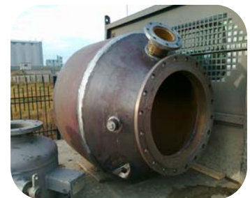
Process vessel operating at 95°C relined using 2 coats of 205 Ceramic HT Fluid
